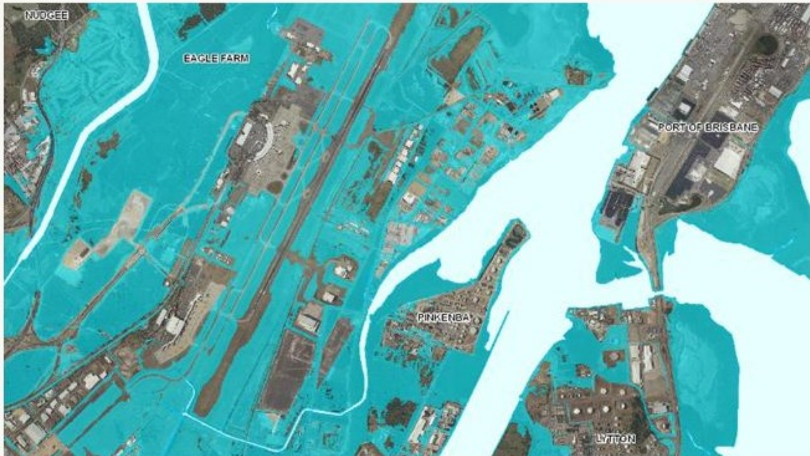
Flood map shows the extent of flooding of Brisbane Airport in 2100 if sea levels rise 1m. Picture: OzCoast, AustralianOnline Coastal Information Source: The Courier-Mail
